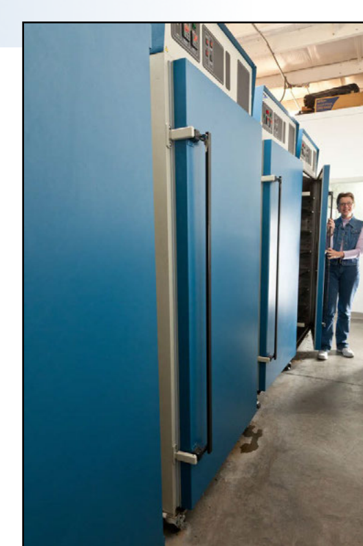
Fig. 8. WIR staff member Barbara Stahl with the Arrhenius ovens maintained at 57, 64, 71, and 78°C—all at 50% RH
