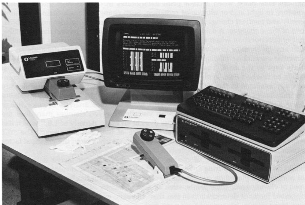
FIG. 5 Density measurements of color print being read with color densitometer (left). Data is entered into microcomputer (center) and recorded on a magnetic "floppy" disc using computer disc drive (right). The computer can be programmed to analyze data in terms of the criterion specified for the densitometric limits of change for color photographs.
