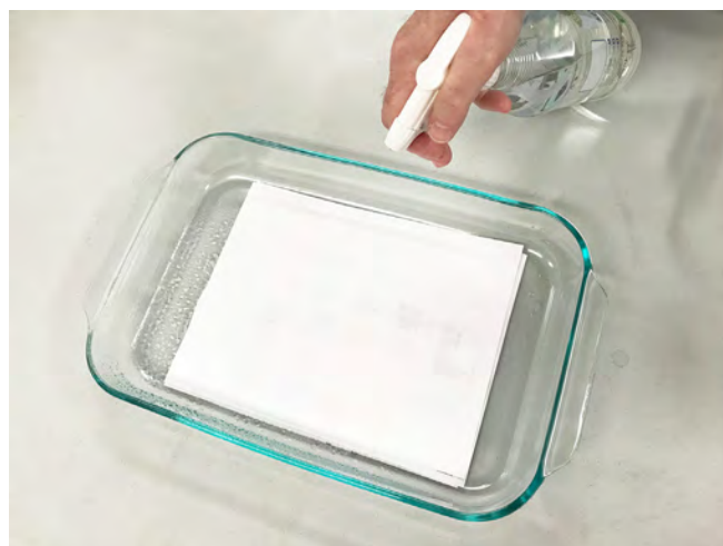
Figure 6. To simulate the effects of immersion in water of multi-page plain paper documents or of multiple pages in a file folder, lightly spraying a blank unprinted sheet with water and then placing a printed test target page on top of it and lightly spraying and, finally, placing another blank page on top of it and spraying it proved to provide better assessments of ink bleeding, ink migration through to the back of the page, and ink transfer to an adjacent page proved to be more meaningful than completely immersing a whole stack of pages in water at the same time.
