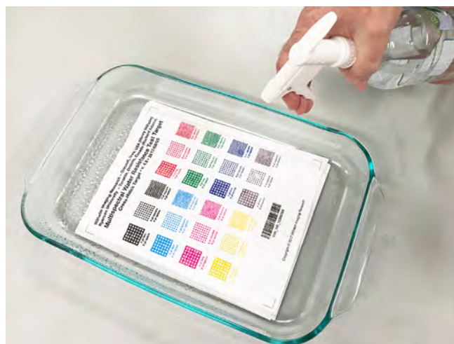
Figure 6. To simulate the effects of immersion in water of multi-page plain paper documents or of multiple pages in a file folder, lightly spraying a blank unprinted sheet with water and then placing a printed test target page on top of it and lightly spraying and, finally, placing another blank page on top of it and spraying it proved to provide better assessments of ink bleeding, ink migration through to the back of the page, and ink transfer to an adjacent page proved to be more meaningful than completely immersing a whole stack of pages in water at the same time.
