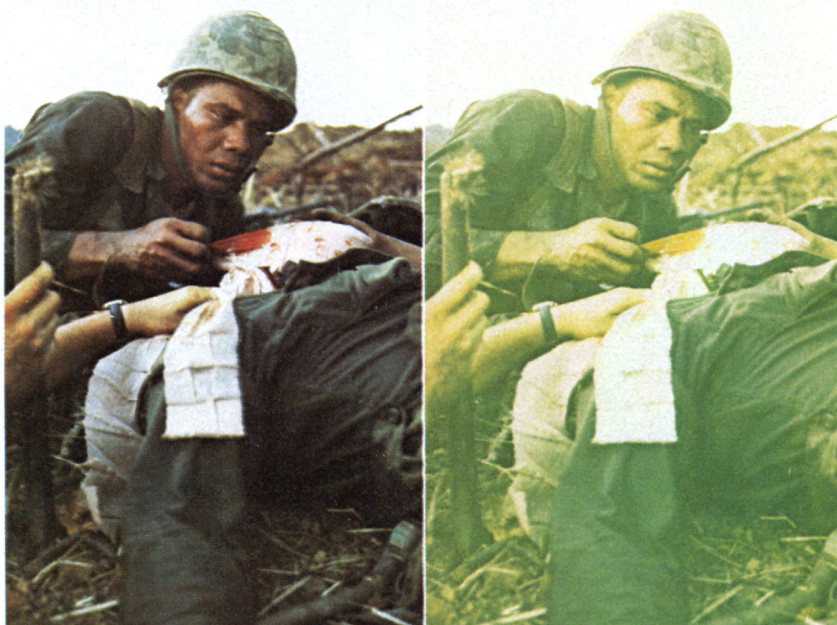
Kodak Ektachrome RC, Type 1993: Shows considerably less stability than Ektacolor above, in overall density and highlight loss. Note cyan dye loss, yellow stain.
