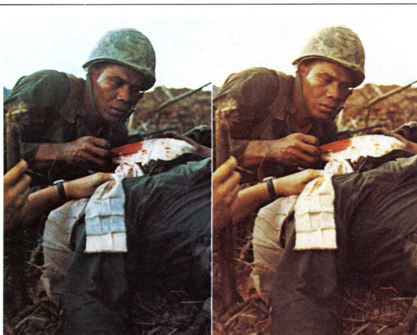
Kodak Ektacolor 74 RC: Note serious losses in overall density and the color shift toward magenta/yellow caused by cyan dye instability under our test conditions.
