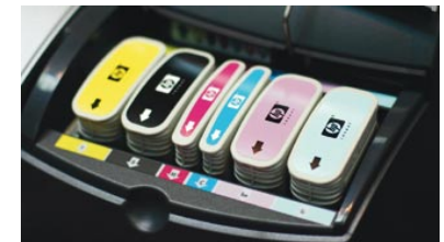
The HP Designjet 130 makes use of six high-stability dye-based photo inks.
