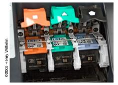
The HP Photosmart 8450 is supplied with three ink cartridges, shown here. In addition, the optional HP No. 94 pigmented black ink cartidge can be used for optimal text quality with plain paper printing.
