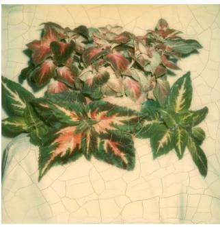
This Polaroid SX-70 print, made in 1972 only a few months after the SX-70 system was introduced, has developed an overall yellowish stain which is plainly evident in the once-white background of this photograph. Cracks can be seen over the whole area of the image; the cracks are located in the image-receiving layer, beneath the transparent polyester print cover sheet. The print has been kept in the dark under normal storage conditions.
