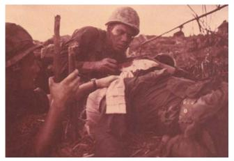
Kodak Ektachrome 22 RC print (initial type: 1984–90) after 6 months in the accelerated dark fading/staining test. Ektachrome Radiance paper (1991—) has greatly improved dye stability in dark storage, but over time the paper still develops high levels of yellowish stain.
