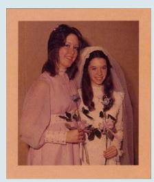
Kodak Ektacolor print after 240 days in an accelerated dark fading/staining test.
