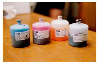
Bottles of the water-base inks employed in the Iris ink jet printers. Initially designed for graphic arts proofing, the standard Iris inks have very poor light fading stability. High-stability inks for fine art and other display applications are expected to become available by the end of 1993.
