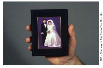
The images of Fuji-Inax Photocera photographs have a screen pattern that can be observed under magnification. Made with a ceramic support, Photocera photographs are fired at high temperatures to fuse the pigment image to the base. Fuji claims the photographs are permanent, even when displayed for many years outdoors in sunlight and rain.
