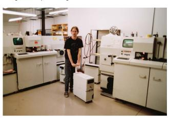
After processing, the spliced rolls of film are printed with Agfa MSP printers. Density and color-balance settings are determined by the computerized printers, each of which can expose between 15,000 and 20,000 prints per hour.
