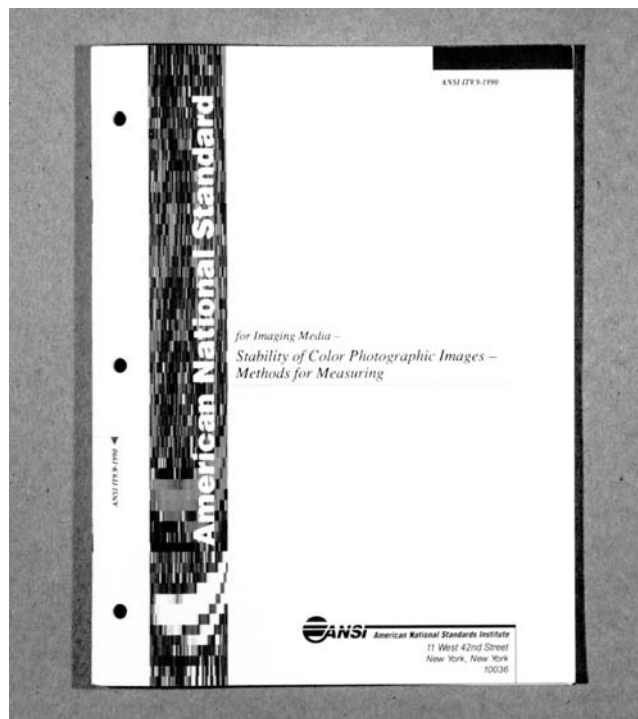
ANSI IT9.9-1990, American National Standard for Imaging Media – Stability of Color Photographic Images – Methods for Measuring specifies a predictive, multi-temperature Arrhenius test for evaluating dark storage stability. The Standard also specifies a number of comparative light fading tests for different display conditions.
