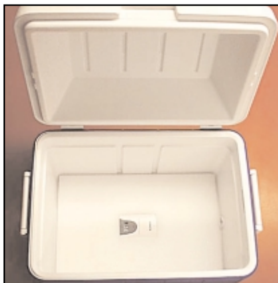
Figure 21. Acclimatisation chamber with wireless thermometer installed.
