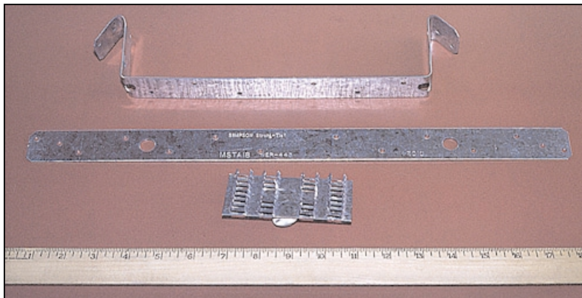
Figure 6. Parts for 'toast rack' mat board drying apparatus. Top: Strap tie bent to form handles. Centre: Strap tie, as purchased. Bottom: Deck mending plate. Wooden rulers were used to lift the hot racks.
